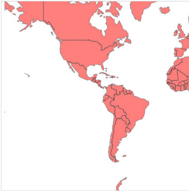
Figure 7.3 A map of the world using the default settings for D3's Mercator projection. You can see most of the Western Hemisphere and some of Europe and Africa, but the rest of the world is rendered out of sight. 🌐
