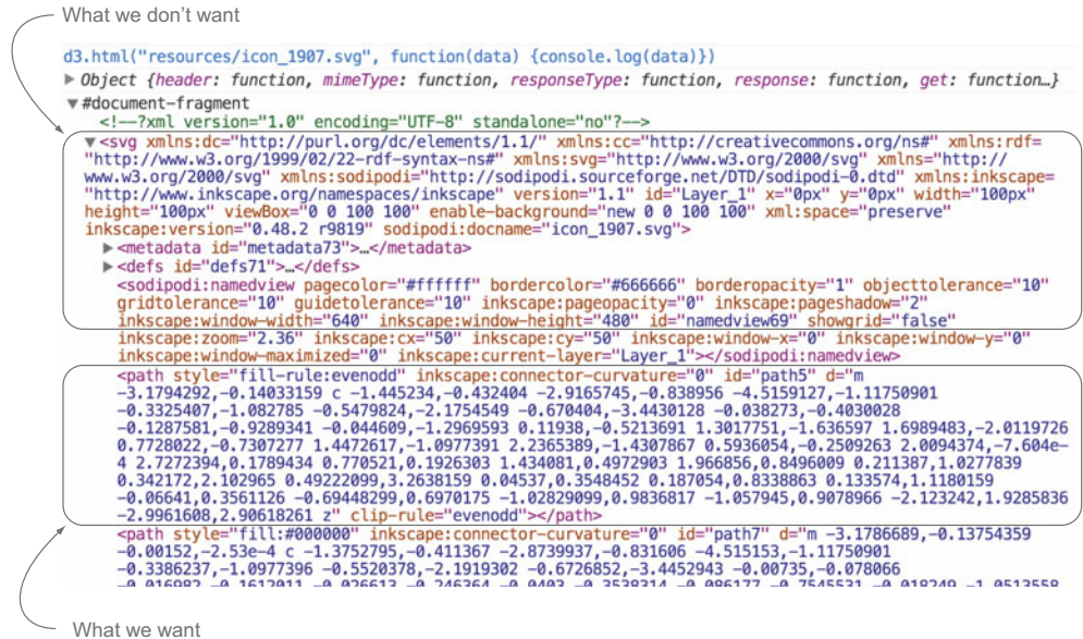
Figure 3.21 An SVG loaded using d3.html() that was created in Inkscape. It consists not only of the graphical <path> elements that make up the SVG but also much data that's often extraneous.
