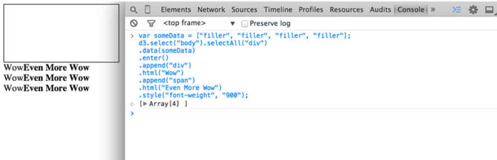
Figure 1.25 By binding an array of four values to a selection of <div> elements on the page, the .enter() function created three new <div> elements to reflect the size mismatch between the data array and the selection. 🎨
