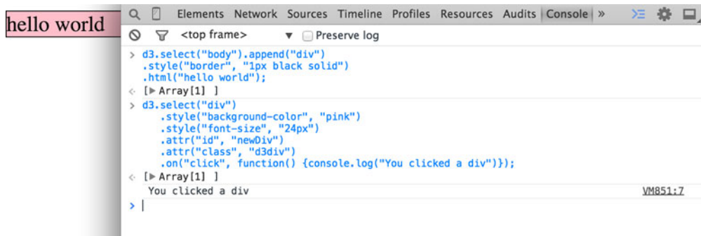
Figure 1.31 Using console.log() , you can test to see if an event is properly firing. Here you create a <div> and assign an onclick event handler using the .on() syntax. When you click that element and fire the event, the action is noted in the console.
